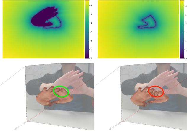
Fig. 3. Visualization of  $\log(DT_{\text{left}} + 1)$  with (top left) and without (top right) occlusion handling. The reconstructed hand without occlusion handling (bottom right) incorrectly articulates to explain an occlusion boundary, while our proposed method (bottom left) correctly handles the occlusion.
